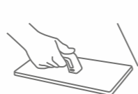
COMPRESSING THE TILE
